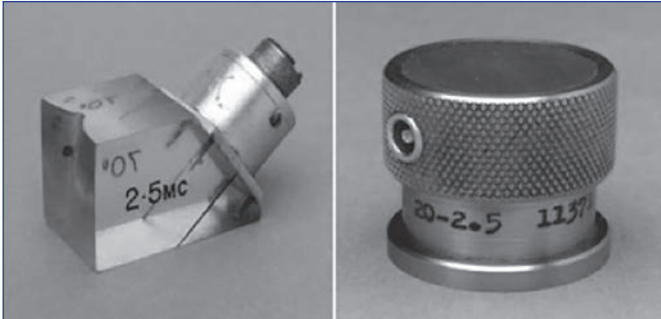
Fig 3. A 2.5MHz 70 degrees shear wave probe and a compression wave probe.
