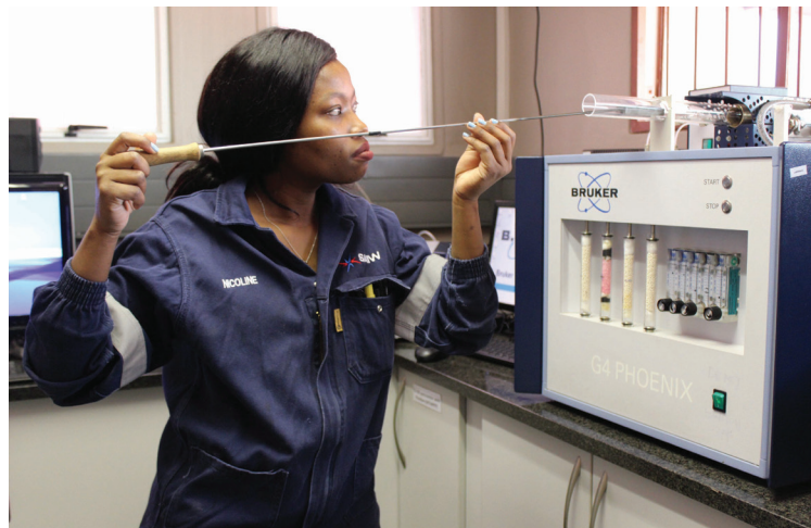
Nicolene Kgoedi SAIW MTL assistant using the Bruker G4 PHOENIX diffusible analyser.
