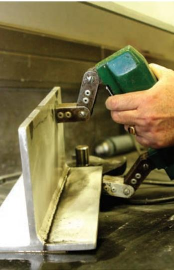
**Magnetic Testing (MT)** – detects surface and slightly subsurface discontinuities in ferromagnetic materials such as iron, nickel, cobalt, and some of their alloys.
