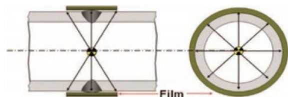
Fig. 2 Single wall, single image (SWSI) or panoramic radiographic technique
