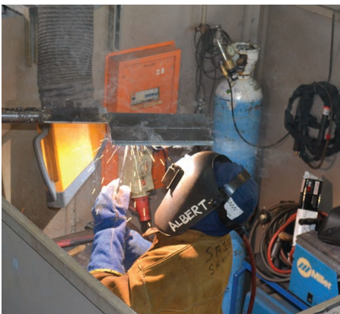
A trainee producing fillet welds on plate in the 4F (overhead) position.
