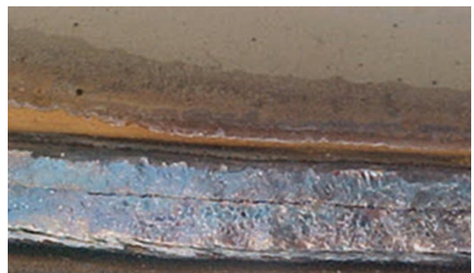
Cold cracks – methods for avoidance
