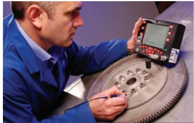
Fig 1 Pen type probe being used to examine bolt holes for cracks.
